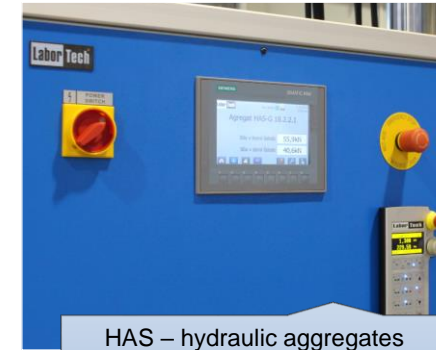
HAS - hydraulic aggregates designed for static tests with integrated diagnostics HALT 16 - Simatic.
