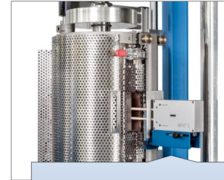
High temperature furnaces up to 1600 ° C.
